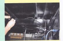
tie wrapping Loop extra wire and use small tiewrap to hold in place Make sure the unused end of hoses are pluged You need an 11/16 & 3/4 wrench Face fittings towards front long hose will go to rear fitting Hose over tube Pictures showing routing of hose Tie hoses together Pictures showing routing of hose over tube, channel, ect.
